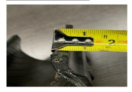
Hook the tape measure to the inside edge of the tire bead and measure the width of the bead, calipers work even better if you have them.
