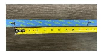
Press masking tape to the inside surface of the tire from bead to bead, as straight as possible. Make sure the tape is making full contact with the inside surface of the tire, and then mark the tape at the INSIDE corners of the beads.
