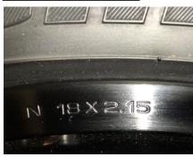
Rim width is typically stamped onto the side of the rim in most modern bikes.
